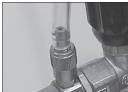
Figure 10 - Attach suction tube to barb fitting
