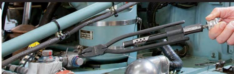
Fast twist in lock-wire securing assemblies subject to vibration.
