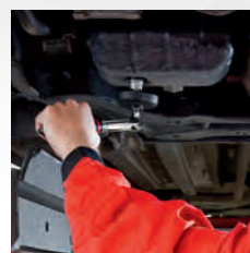
1 Drain plug unlocking in power position.
