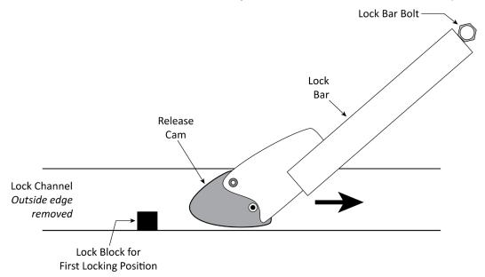
Not necessarily to scale. Not all components shown. Release Cam and the Lock Bar shown moving off of the First Locking Position towards the Top Locking Position.
