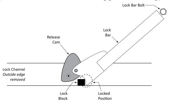
Not necessarily to scale. Not all components shown. Shows Release Cam and Lock Bar in Locked Position.
