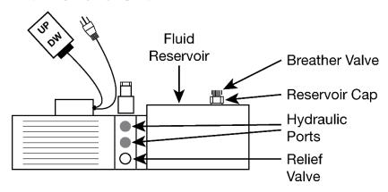
Drawing not necessarily to scale. Some Power Units may be slightly different.
