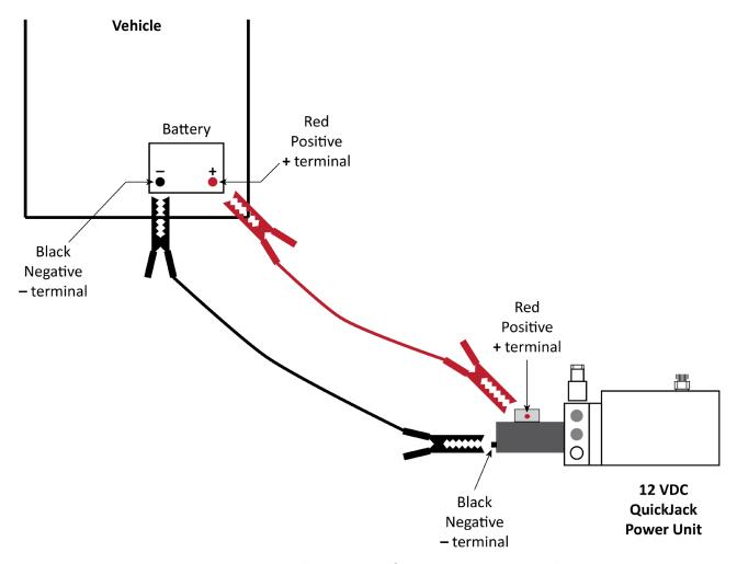
Not to scale. Not all components shown. The Jumper Cables and the Vehicle Battery are not supplied with the 12 VDC QuickJack Power Unit.
