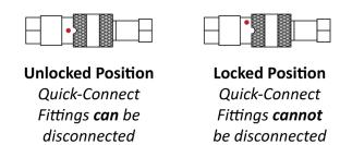
**To lock a connection**: Push the Male Quick-Connect Fitting into the Female Quick-Connect Fitting, then turn the Moveable Section so that the Lock Ball is not opposite the Notch.
