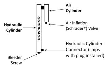
The components of the Air and Hydraulic Cylinders are:
