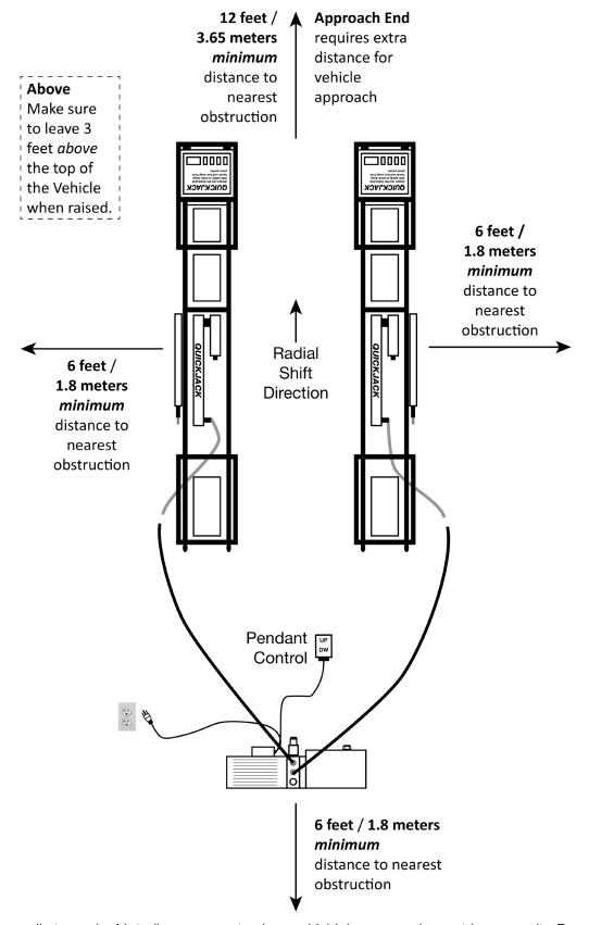
Not necessarily to scale. Not all components shown. Vehicle approach must be opposite Power Unit. Do not drive Vehicle on Hydraulic Hoses, Power Unit, or QuickJack Frames.
