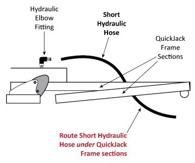
Drawing not necessarily to scale. Not all components shown, some exaggerated for clarity. Hydraulic Elbow Fitting is shown pointed up for clarity; it is not actually installed this way.
