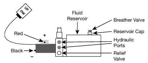
Drawing not necessarily to scale. Some Power Units may be slightly different.
