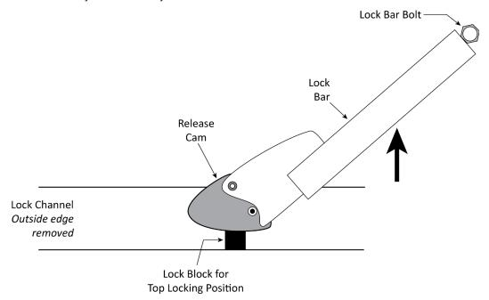
Not necessarily to scale. Not all components shown. Release Cam shown on top of the Lock Block for the Top Locking Position.
