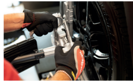
Single fast-action knob for easy clamping
